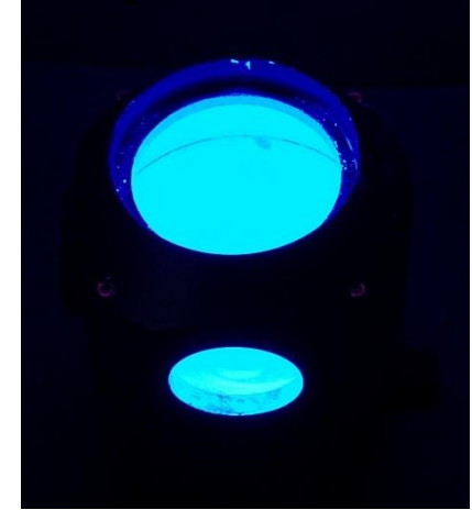
\text{BaMgAl}_{10}\text{O}_{17}:\text{Eu} coated integration sphere under daylight or upon VUV exc.
