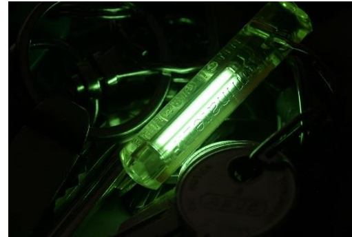
Tritium filled tube coated with \text{Zn}_2\text{SiO}_4:\text{Mn}^{2+}
