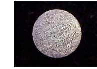
IR-Ref-Al1-80 80 grade abrasive paper 190 \mu\text{m} granulation
