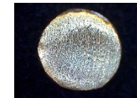
IR-Ref-Au1-80 80 grade abrasive paper 190 \mu\text{m} granulation
